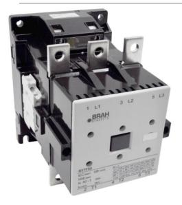
**PART NUMBER – B3TF5522-0AK6**: BRAH Electric, aftermarket direct replacement contactors for Siemens 3TF5522-0AK6, World Series, type 3TF, 3P, 3PH, 300A, 600V, 125HP @ 230V, 250HP @ 460V, 300HP @ 575V, complete with 110/120V AC coil, 2 N/O - 2 N/C auxiliary contact, AC magnetic contactor, suitable for use with 3TF series motor control systems
