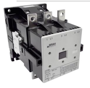
**PART NUMBER – B3TF5622-0AK6**: BRAH Electric, aftermarket direct replacement contactors for Siemens 3TF5622-0AK6, World Series, type 3TF, 3P, 3PH, 400A, 600V, 150HP @ 230V, 300HP @ 460V, 400HP @ 575V, complete with 110/120V AC coil, 2 N/O - 2 N/C auxiliary contact, AC magnetic contactor, suitable for use with 3TF series motor control systems
