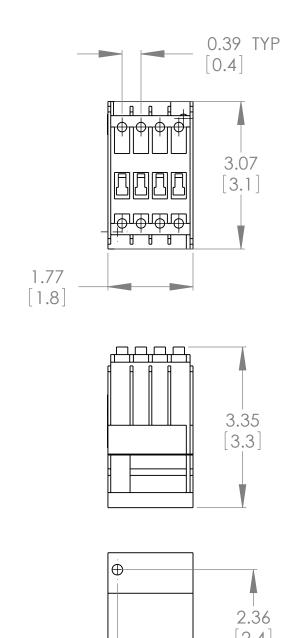
\* NOTE: BRAH ELECTRIC CONTACTOR B3TH4022 IS AN AFTERMARKET DIRECT REPLACMENT FOR SEIMENS 3TH4022, 3TH SERIES. SUITABLE FOR USE WITH 3TH SERIES MOTOR CONTROL SYSTEMS
