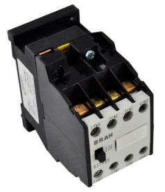
**PART NUMBER – B3TH80:** BRAH Electric, aftermarket direct replacement contactors for Siemens 3TH80, World Series, type 3TH, 4P, 3PH, 16A, 600V, complete with 120V AC coil, 2 N/O - 2 N/C auxiliary contact, AC magnetic contactor, suitable for use with 3TH series motor control systems
