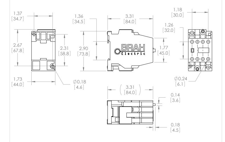
\* NOTE: BRAH ELECTRIC CONTACTOR B3TH 8244 IS AN AFTERMARKET DIRECT REPLACMENT FOR SEIMENS 3TH8244,3TH SERIES. SUITABLE FOR USE WITH 3TH SERIES MOTOR CONTROL SYSTEMS
