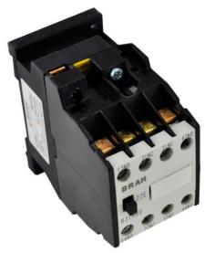
MAGNETIC CONTACTOR PART NO. B3TH8244 <u>PART NUMBER – B3TH8244</u>: BRAH Electric, aftermarket direct replacement contactors for Siemens 3TH8244, World Series, type 3TH, 3P, 3PH, 16A, 600V, complete with 120V AC coil, 2 N/O - 2 N/C auxiliary contact, AC magnetic contactor, suitable for use with 3TH series motor control systems
