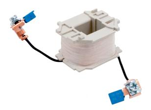
**PART NUMBER - B3TY7403-0AU1:** BRAH Electric, aftermarket direct replacement coils for Siemens 3TY7403-0AU1, World Series, type B3TY7, 277VAC 60Hz, suitable for use with 3TF30, 3TF31, 3TF32, 3TF33, 3TF40, 3TF41, 3TF42, 3TF43 contactors.
