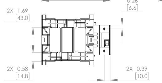
\* NOTE: BRAH ELECTRIC COILS ARE A DIRECT REPLACEMENT FOR SIEMENS 3TY7503-0AP6, WORLD SERIES, TYPE B3TY7, 24V AC 60HZ, SUITABLE FOR USE WITH 3TF50, 3TF51 CONTACTORS
