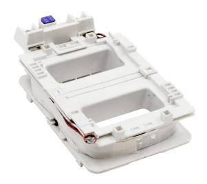
**PART NUMBER - B3TY7523-OAK6:** BRAH Electric, aftermarket direct replacement coils for Siemens 3TY7523-OAK6, World Series, type B3TY7, 120V AC 60Hz, suitable for use with 3TF52, 3TF53 contactors
