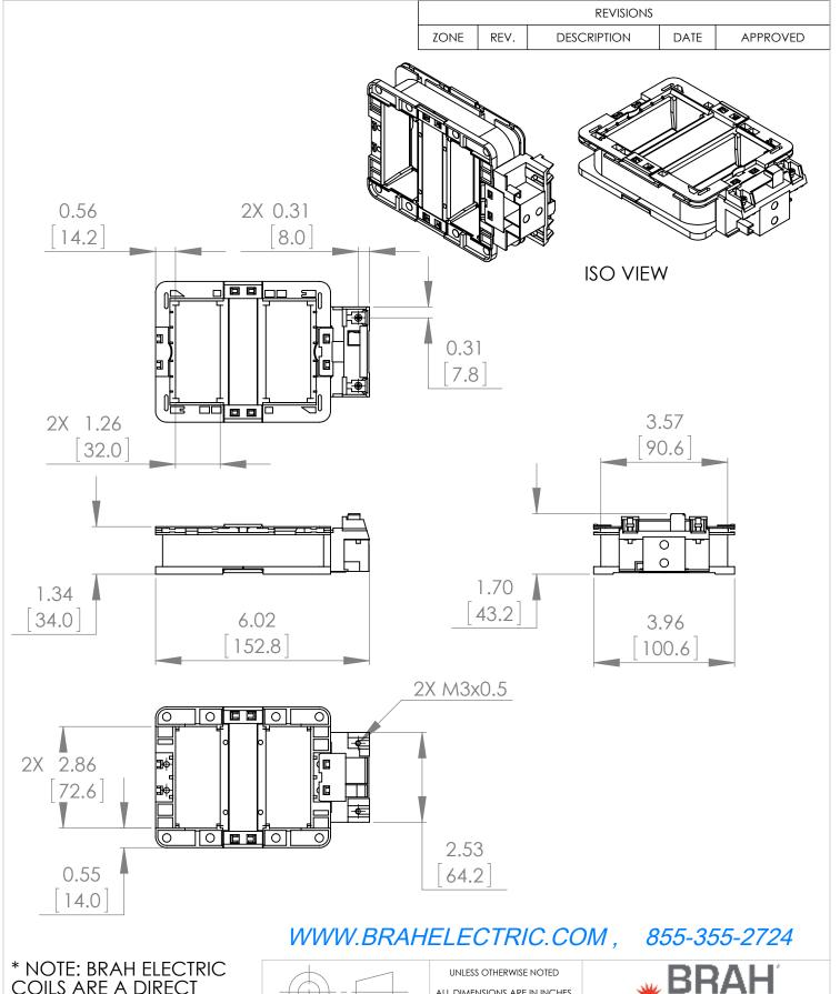
COILS ARE A DIRECT REPLACEMENT FOR SIEMENS 3TY7563-0AK6, WORLD SERIES, TYPE B3TY7, 120V AC 60HZ, SUITABLE FOR USE WITH 3TF56 CONTACTORS
