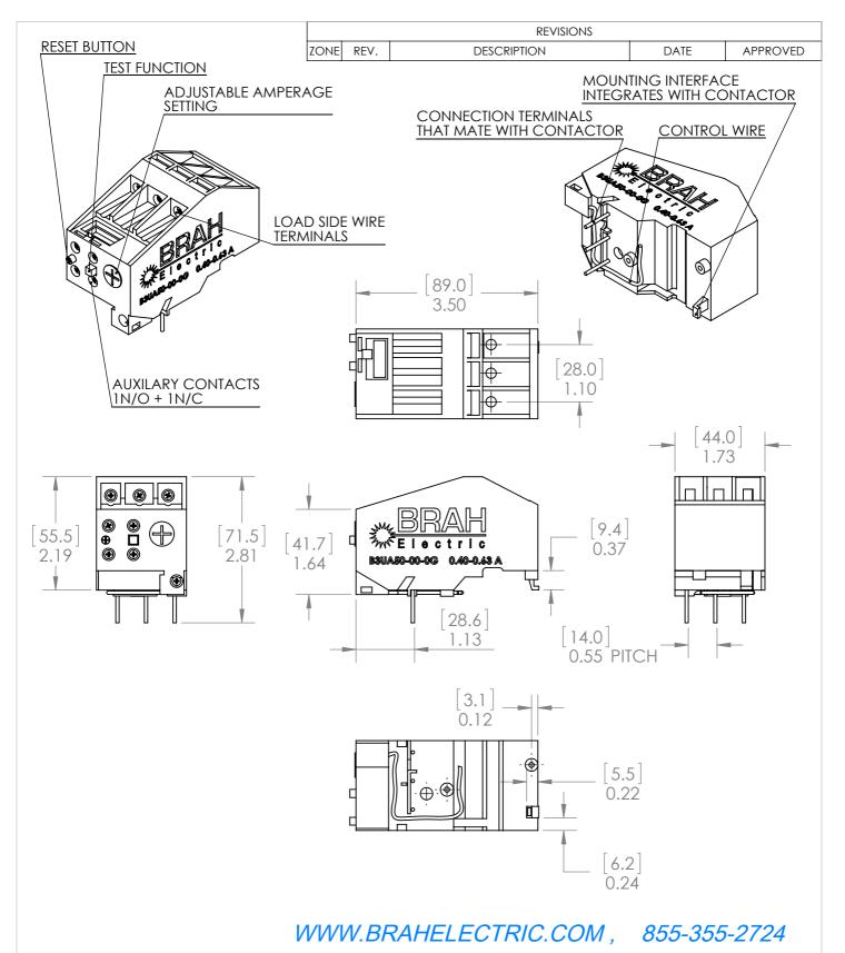
\*NOTE: THIS BRAH ELECTRIC OVERLOAD RELAY B3UA50-00-0G AN AFTERMARKET DIRECT REPLACMENT FOR SIEMENS 3UA50-00-0G. SUITABLE FOR USE WITH 3UA MOTOR CONTROL SYSTEMS
