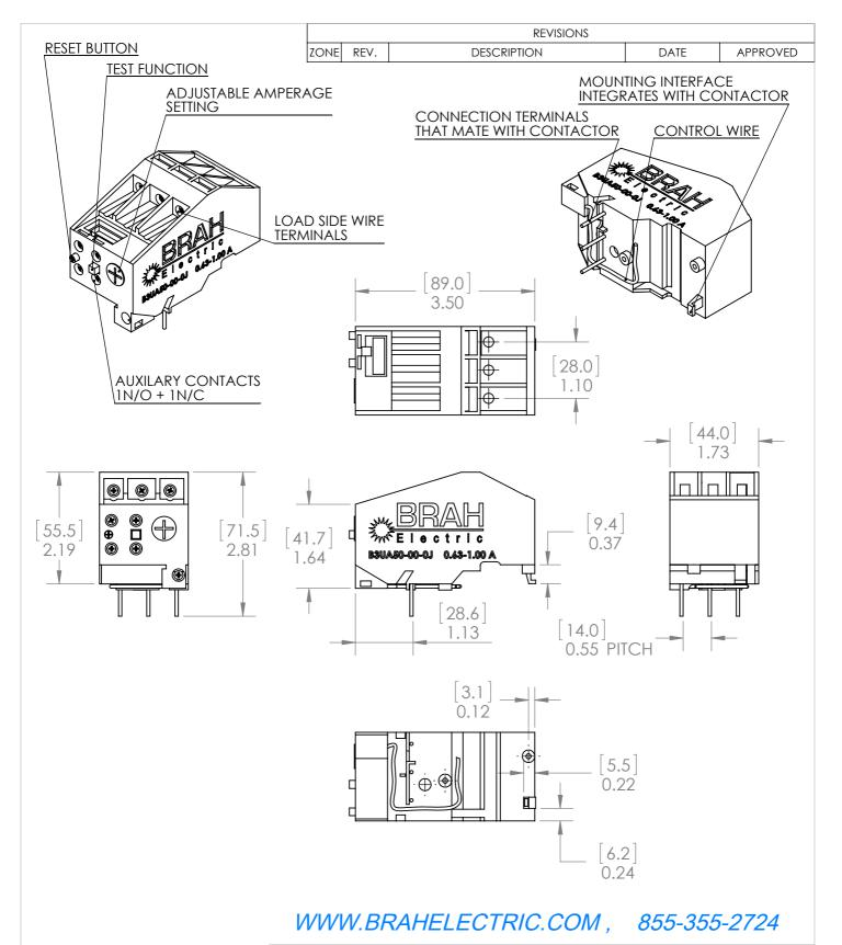
\*NOTE: THIS BRAH ELECTRIC OVERLOAD RELAY B3UA50-00-0J AN AFTERMARKET DIRECT REPLACMENT FOR SIEMENS 3UA50-00-0J. SUITABLE FOR USE WITH 3UA MOTOR CONTROL SYSTEMS
