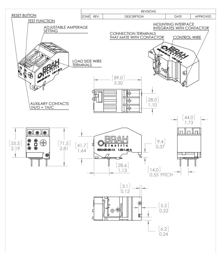
\*NOTE: THIS BRAH ELECTRIC **OVERLOAD RELAY** B3UA50-00-1A AN AFTERMARKET DIRECT REPLACMENT FOR SIEMENS 3UA50-00-1A. SUITABLE FOR USE WITH 3UA MOTOR CONTROL SYSTEMS
