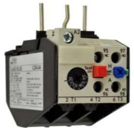
PARTNUMBER-B3UA50-00-1B: BRAH Electric, aftermarket direct replacement solid state overload relays for Siemens 3UA50-00-1B, World Series, type 3UA, rated for 1.25-2.00 amps, suitable for 3TF30, 3TF31, 3TF40, 3TF41, 3TB40, 3TB41 contactors
