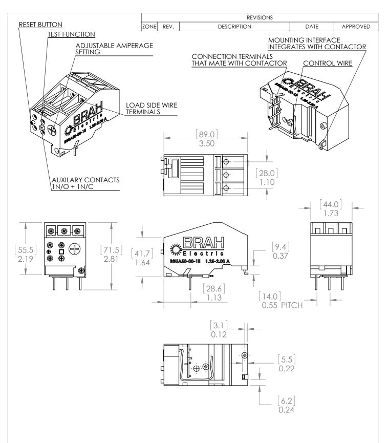
\*NOTE: THIS BRAH ELECTRIC **OVERLOAD RELAY** B3UA50-00-1B AN AFTERMARKET DIRECT REPLACMENT FOR SIEMENS 3UA50-00-1B. SUITABLE FOR USE WITH 3UA MOTOR CONTROL SYSTEMS
