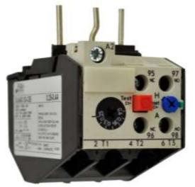
PART NUMBER – B3UA50-00-1E: BRAH Electric, aftermarket direct replacement solid state overload relays for Siemens 3UA50-00-1E, World Series, type 3UA, rated for 2.50-4.00 amps, suitable for 3TF30, 3TF31, 3TF40, 3TF41, 3TB40, 3TB41 contactors
