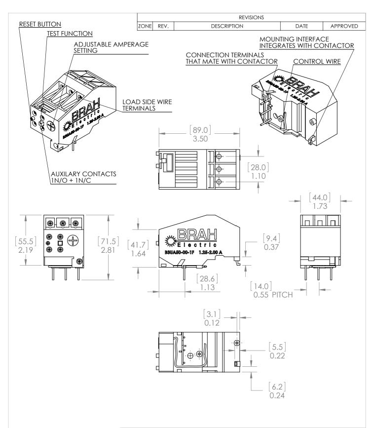
\*NOTE: THIS BRAH ELECTRIC **OVERLOAD RELAY** B3UA50-00-1F AN AFTERMARKET DIRECT REPLACMENT FOR SIEMENS 3UA50-00-1F. SUITABLE FOR USE WITH 3UA MOTOR CONTROL SYSTEMS
