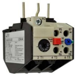
PART NUMBER – B3UA50-00-1K: BRAH Electric, aftermarket direct replacement solid state overload relays for Siemens 3UA50-00-1K, World Series, type 3UA, rated for 8.00-12.50 amps, suitable for 3TF30, 3TF31, 3TF40, 3TF41, 3TB40, 3TB41 contactors
