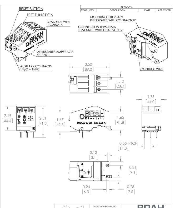
\*NOTE: THIS BRAH ELECTRIC OVERLOAD RELAY B3UA52-00-0C AN AFTERMARKET DIRECT REPLACMENT FOR SIEMENS 3UA52-00-0C. SUITABLE FOR USE WITH 3UA MOTOR CONTROL SYSTEMS
