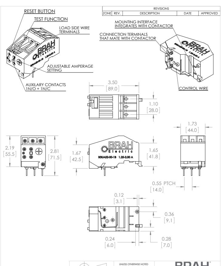
\*NOTE: THIS BRAH ELECTRIC **OVERLOAD RELAY** B3UA52-00-1B AN AFTERMARKET DIRECT REPLACMENT FOR SIEMENS 3UA52-00-1B. SUITABLE FOR USE WITH 3UA MOTOR **CONTROL SYSTEMS**
