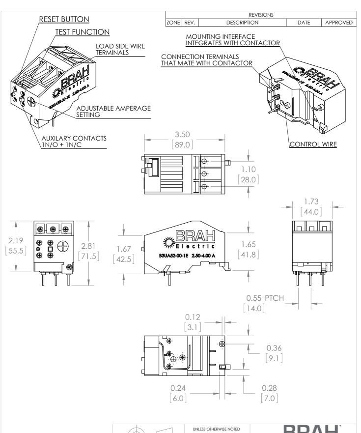
\*NOTE: THIS BRAH ELECTRIC OVERLOAD RELAY B3UA52-00-1E AN AFTERMARKET DIRECT REPLACMENT FOR SIEMENS 3UA52-00-1E. SUITABLE FOR USE WITH 3UA MOTOR CONTROL SYSTEMS
