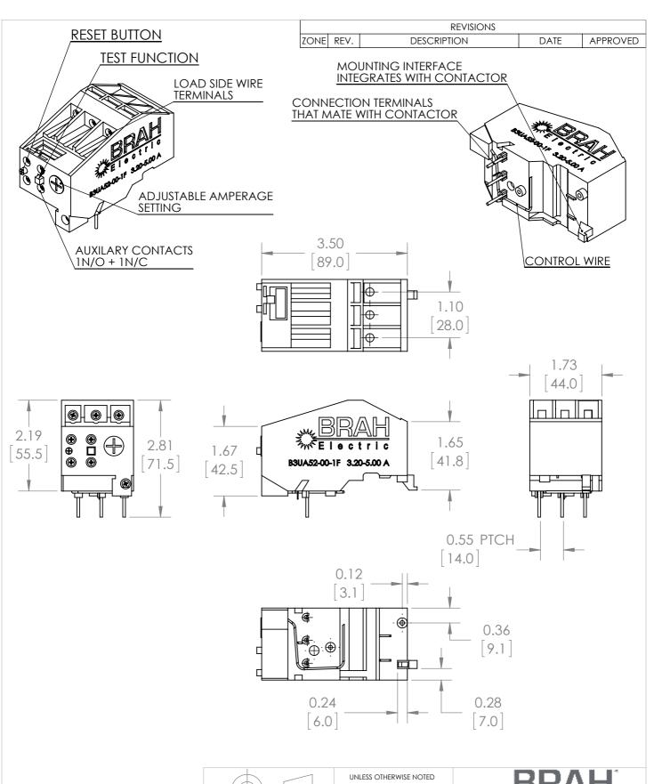
\*NOTE: THIS BRAH ELECTRIC OVERLOAD RELAY B3UA52-00-1F AN AFTERMARKET DIRECT REPLACMENT FOR SIEMENS 3UA52-00-1F. SUITABLE FOR USE WITH 3UA MOTOR CONTROL SYSTEMS
