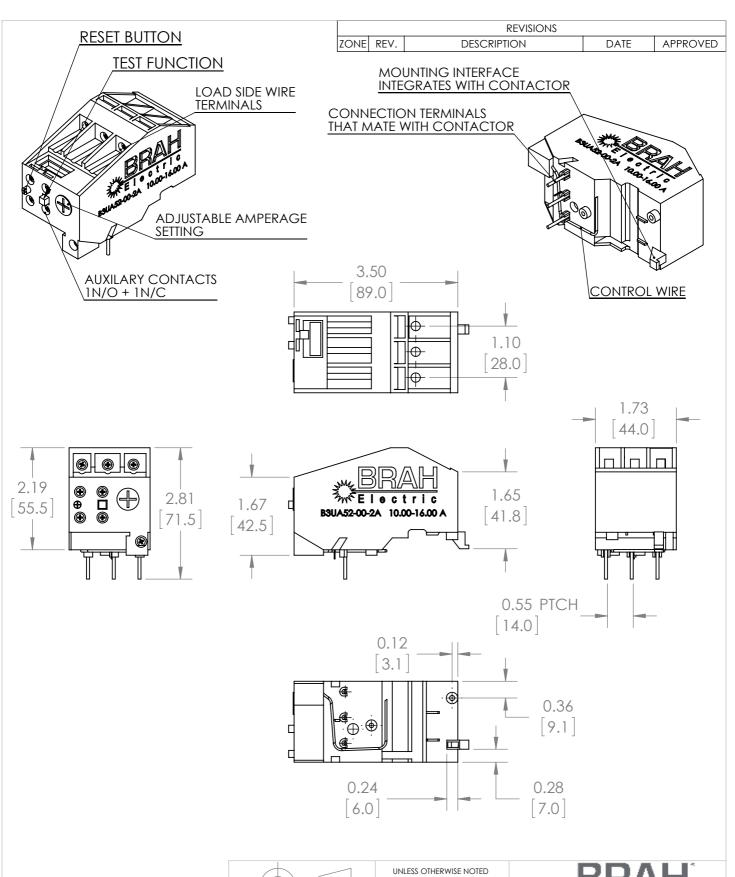
\*NOTE: THIS BRAH ELECTRIC **OVERLOAD RELAY** B3UA52-00-2A AN AFTERMARKET DIRECT REPLACMENT FOR SIEMENS 3UA52-00-2A. SUITABLE FOR USE WITH 3UA MOTOR **CONTROL SYSTEMS**
