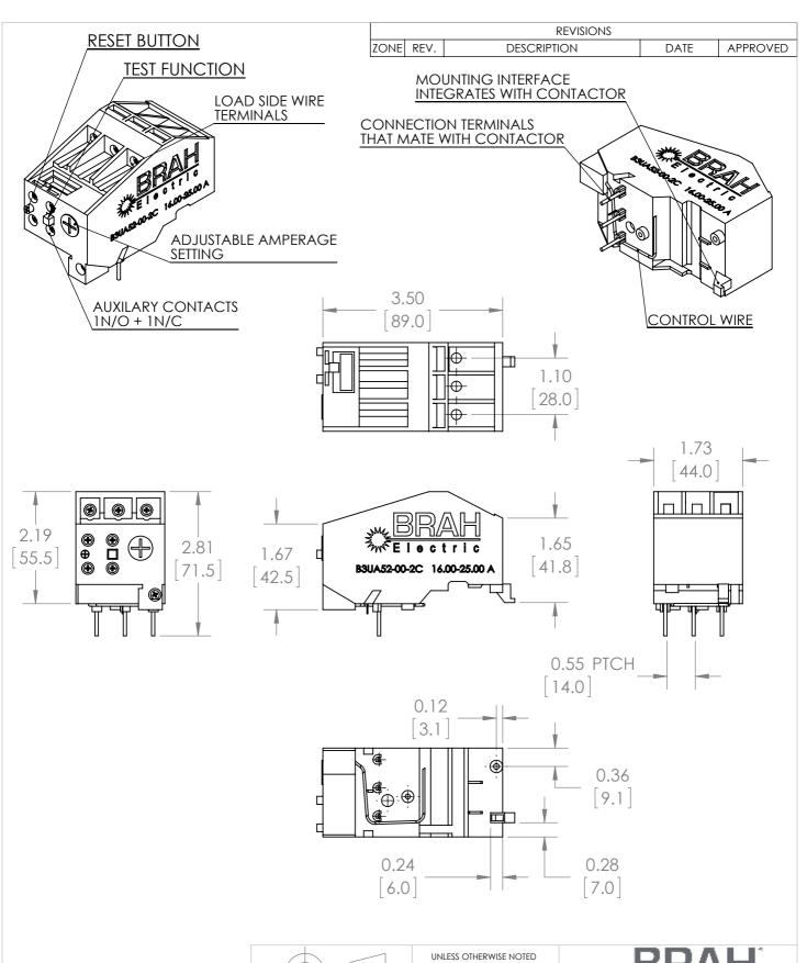
\*NOTE: THIS BRAH ELECTRIC **OVERLOAD RELAY** B3UA52-00-2C AN AFTERMARKET DIRECT REPLACMENT FOR SIEMENS 3UA52-00-2C. SUITABLE FOR USE WITH 3UA MOTOR **CONTROL SYSTEMS**
