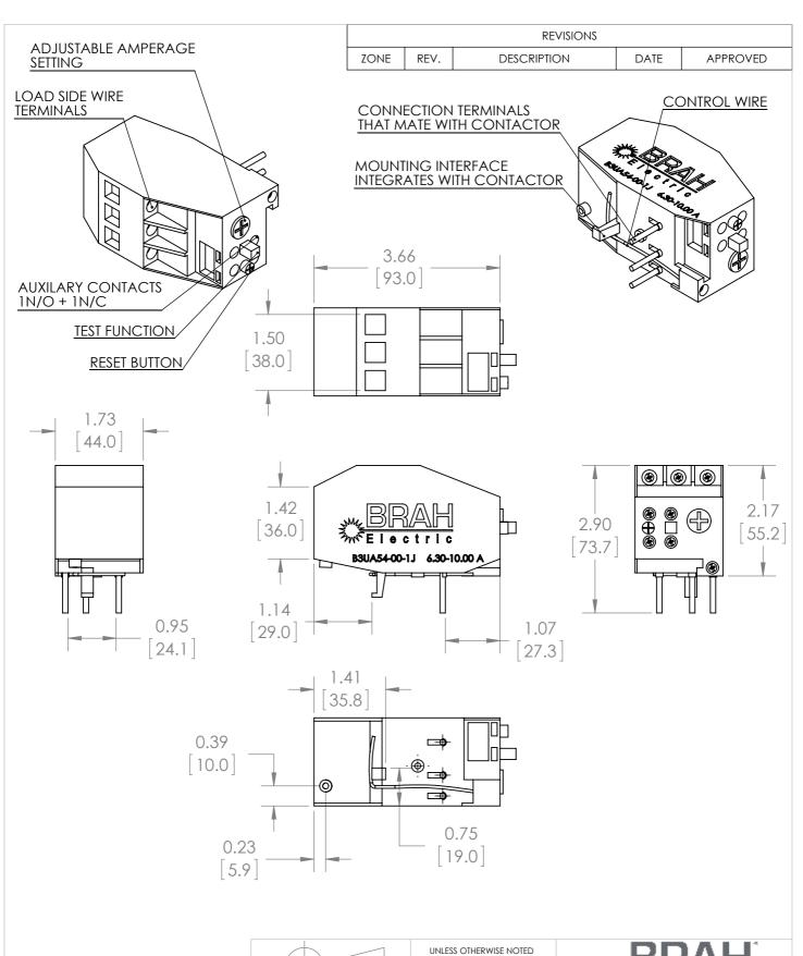
\*NOTE: THIS BRAH ELECTRIC **OVERLOAD RELAY** B3UA54-00-1J AN AFTERMARKET DIRECT REPLACMENT FOR SIEMENS 3UA54-00-1J. SUITABLE FOR USE WITH 3UA MOTOR CONTROL SYSTEMS
