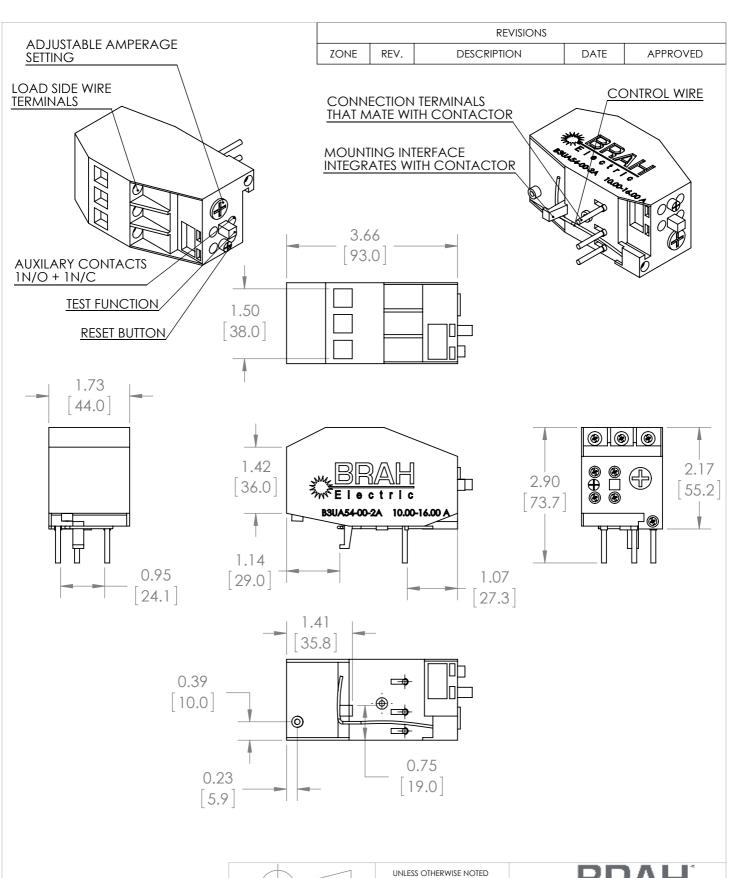
\*NOTE: THIS BRAH ELECTRIC **OVERLOAD RELAY** B3UA54-00-2A AN AFTERMARKET DIRECT REPLACMENT FOR SIEMENS 3UA54-00-2A. SUITABLE FOR USE WITH 3UA MOTOR CONTROL SYSTEMS
