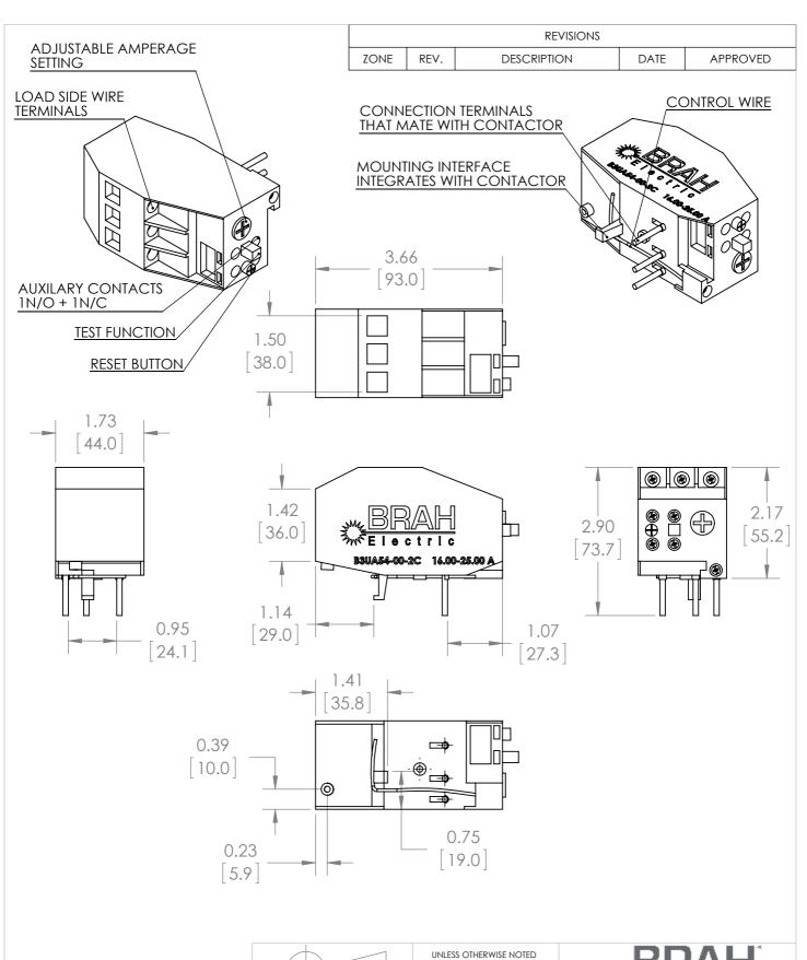
\*NOTE: THIS BRAH ELECTRIC **OVERLOAD RELAY** B3UA54-00-2C AN AFTERMARKET DIRECT REPLACMENT FOR SIEMENS 3UA54-00-2C. SUITABLE FOR USE WITH 3UA MOTOR CONTROL SYSTEMS
