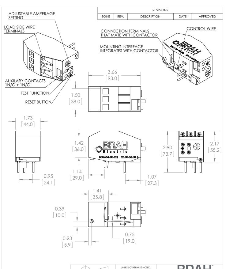
\*NOTE: THIS BRAH ELECTRIC **OVERLOAD RELAY** B3UA54-00-2Q AN AFTERMARKET DIRECT REPLACMENT FOR SIEMENS 3UA54-00-2Q. SUITABLE FOR USE WITH 3UA MOTOR CONTROL SYSTEMS
