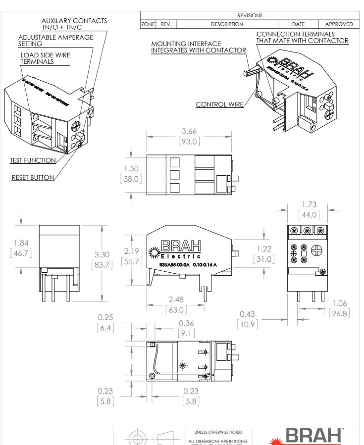
\*NOTE: THIS BRAH ELECTRIC **OVERLOAD RELAY** B3UA55-00-0A AN AFTERMARKET DIRECT REPLACMENT FOR SIEMENS 3UA55-00-0A. SUITABLE FOR USE WITH 3UA MOTOR **CONTROL SYSTEMS**
