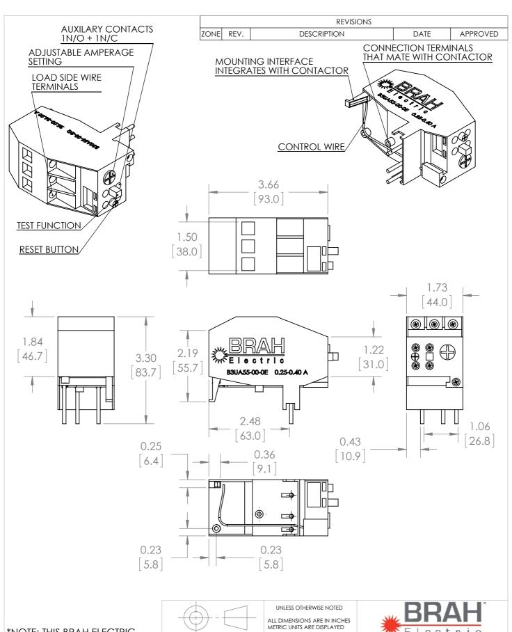
\*NOTE: THIS BRAH ELECTRIC **OVERLOAD RELAY** B3UA55-00-0E AN AFTERMARKET DIRECT REPLACMENT FOR SIEMENS 3UA55-00-0E. SUITABLE FOR USE WITH 3UA MOTOR **CONTROL SYSTEMS**
