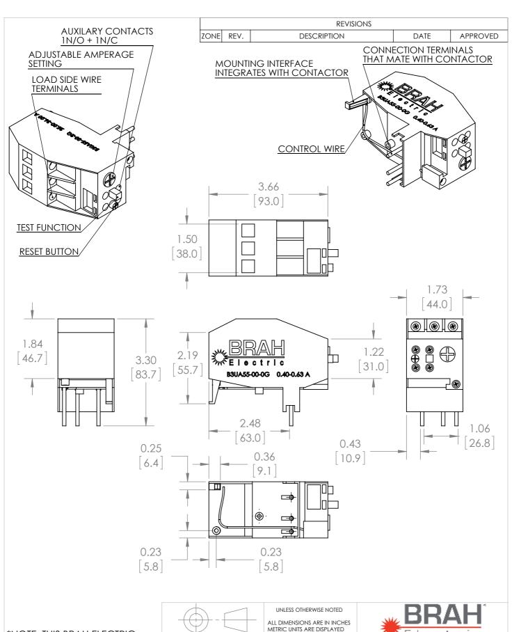
\*NOTE: THIS BRAH ELECTRIC **OVERLOAD RELAY** B3UA55-00-0G AN AFTERMARKET DIRECT REPLACMENT FOR SIEMENS 3UA55-00-0G. SUITABLE FOR USE WITH 3UA MOTOR **CONTROL SYSTEMS**
