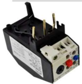
PART NUMBER - B3UA55-00-0G: BRAH Electric, aftermarket direct replacement solid state overload relays for Siemens 3UA55-00-0G, World Series, type 3UA, rated for 0.40-0.63 amps, suitable for 3TF34, 3TF35, 3TF44, 3TF45 contactors
