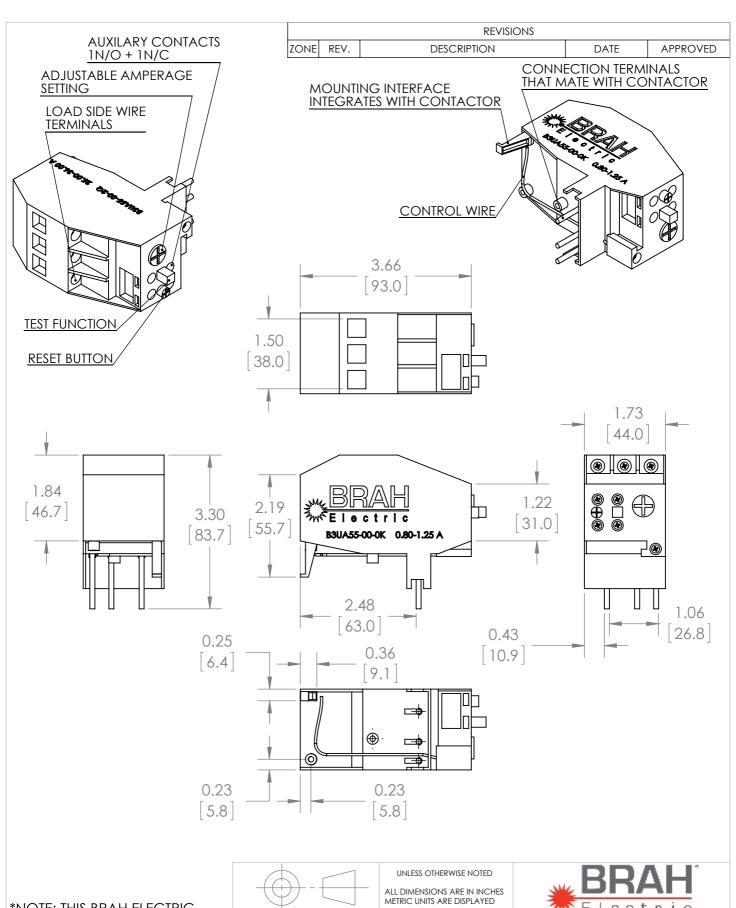
\*NOTE: THIS BRAH ELECTRIC **OVERLOAD RELAY** B3UA55-00-0K AN AFTERMARKET DIRECT REPLACMENT FOR SIEMENS 3UA55-00-0K, SUITABLE FOR USE WITH 3UA MOTOR **CONTROL SYSTEMS**
