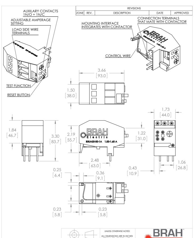
\*NOTE: THIS BRAH ELECTRIC **OVERLOAD RELAY** B3UA55-00-1A AN AFTERMARKET DIRECT REPLACMENT FOR SIEMENS 3UA55-00-1A. SUITABLE FOR USE WITH 3UA MOTOR **CONTROL SYSTEMS**
