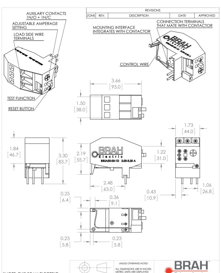
\*NOTE: THIS BRAH ELECTRIC **OVERLOAD RELAY** B3UA55-00-1D AN AFTERMARKET DIRECT REPLACMENT FOR SIEMENS 3UA55-00-1D. SUITABLE FOR USE WITH 3UA MOTOR **CONTROL SYSTEMS**
