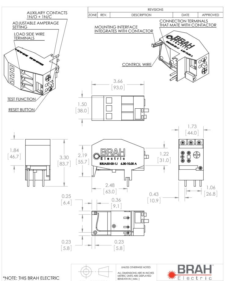
**OVERLOAD RELAY** B3UA55-00-2Q AN AFTERMARKET DIRECT REPLACMENT FOR SIEMENS 3UA55-00-2Q. SUITABLE FOR USE WITH 3UA MOTOR **CONTROL SYSTEMS**
