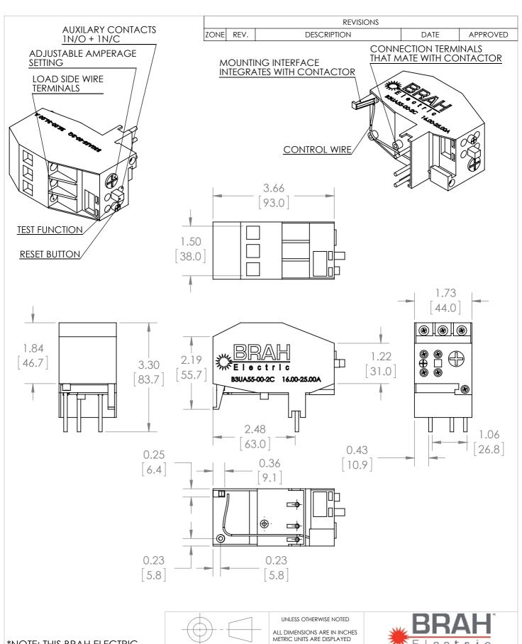
\*NOTE: THIS BRAH ELECTRIC **OVERLOAD RELAY** B3UA55-00-2C AN AFTERMARKET DIRECT REPLACMENT FOR SIEMENS 3UA55-00-2C. SUITABLE FOR USE WITH 3UA MOTOR **CONTROL SYSTEMS**
