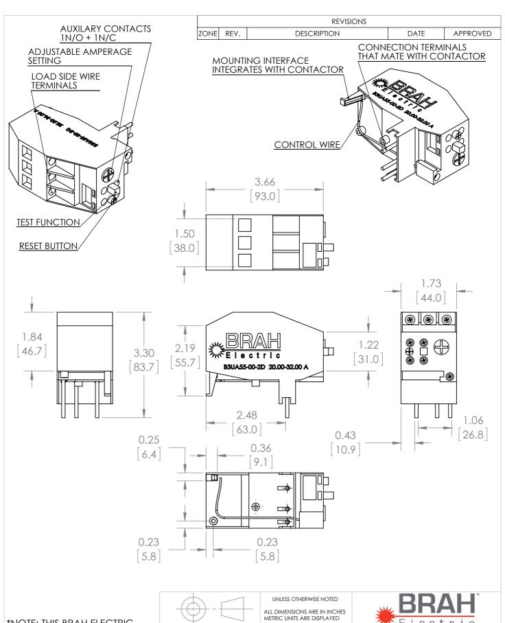
\*NOTE: THIS BRAH ELECTRIC **OVERLOAD RELAY** B3UA55-00-2D AN AFTERMARKET DIRECT REPLACMENT FOR SIEMENS 3UA55-00-2D. SUITABLE FOR USE WITH 3UA MOTOR **CONTROL SYSTEMS**
