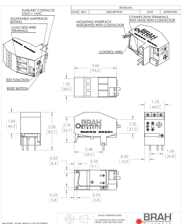
\*NOTE: THIS BRAH ELECTRIC **OVERLOAD RELAY** B3UA55-00-2Q AN AFTERMARKET DIRECT REPLACMENT FOR SIEMENS 3UA55-00-2Q. SUITABLE FOR USE WITH 3UA MOTOR **CONTROL SYSTEMS**
