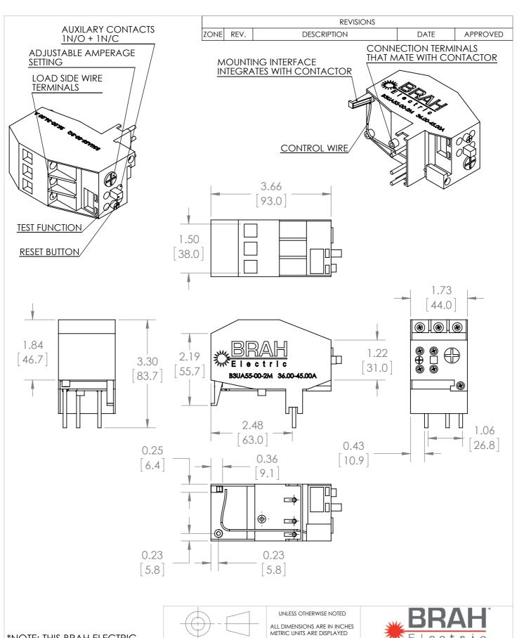
\*NOTE: THIS BRAH ELECTRIC **OVERLOAD RELAY** B3UA55-00-2M AN AFTERMARKET DIRECT REPLACMENT FOR SIEMENS 3UA55-00-2M. SUITABLE FOR USE WITH 3UA MOTOR **CONTROL SYSTEMS**
