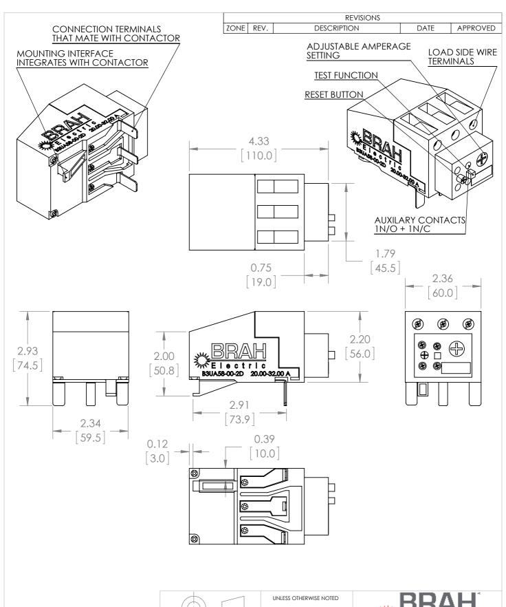
\* NOTE: THIS BRAH ELECTRIC OVERLOAD RELAY B3UA58-00-2D AN AFTERMARKET DIRECT REPLACMENT FOR SIEMENS 3UA58-00-2D. SUITABLE FOR USE WITH 3UA MOTOR CONTROL SYSTEMS
