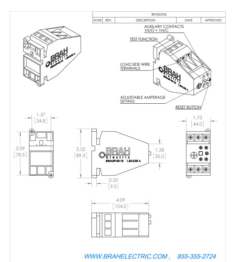
\*NOTE: THIS BRAH ELECTRIC OVERLOAD RELAY B3UA59-00-1B AN AFTERMARKET DIRECT REPLACMENT FOR SIEMENS 3UA59-00-1B. SUITABLE FOR USE WITH 3UA MOTOR CONTROL SYSTEMS
