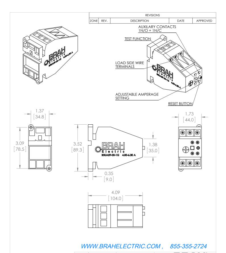
\*NOTE: THIS BRAH ELECTRIC **OVERLOAD RELAY** B3UA59-00-1G AN AFTERMARKET DIRECT REPLACMENT FOR SIEMENS 3UA59-00-1G. SUITABLE FOR USE WITH 3UA MOTOR CONTROL SYSTEMS
