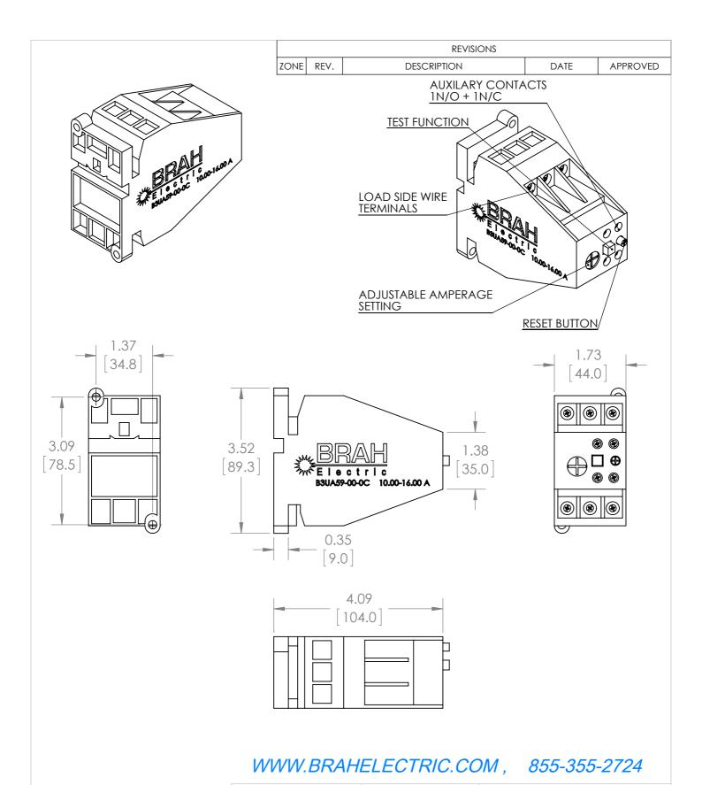
\*NOTE: THIS BRAH ELECTRIC OVERLOAD RELAY B3UA59-00-1 J AN AFTERMARKET DIRECT REPLACMENT FOR SIEMENS 3UA59-00-1 J. SUITABLE FOR USE WITH 3UA MOTOR CONTROL SYSTEMS
