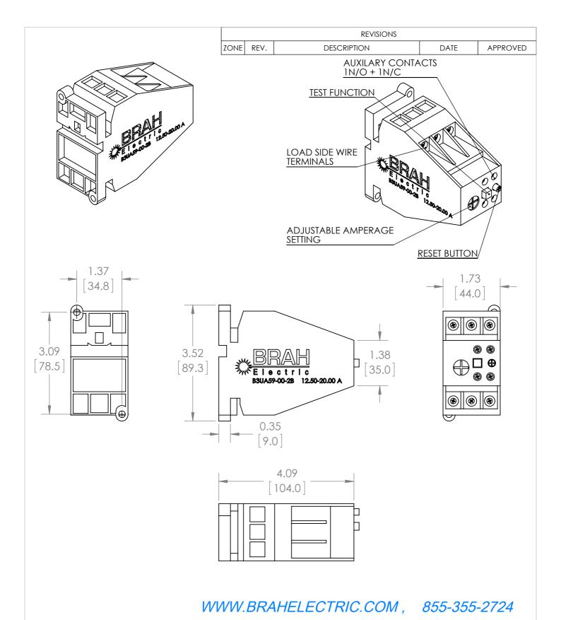
\*NOTE: THIS BRAH ELECTRIC OVERLOAD RELAY B3UA59-00-2B AN AFTERMARKET DIRECT REPLACMENT FOR SIEMENS 3UA59-00-2B. SUITABLE FOR USE WITH 3UA MOTOR CONTROL SYSTEMS
