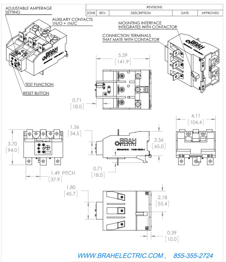
\*NOTE: THIS BRAH ELECTRIC OVERLOAD RELAY B3UA60-00-3J AN AFTERMARKET DIRECT REPLACMENT FOR SIEMENS 3UA60-00-3J. SUITABLE FOR USE WITH 3UA MOTOR CONTROL SYSTEMS
