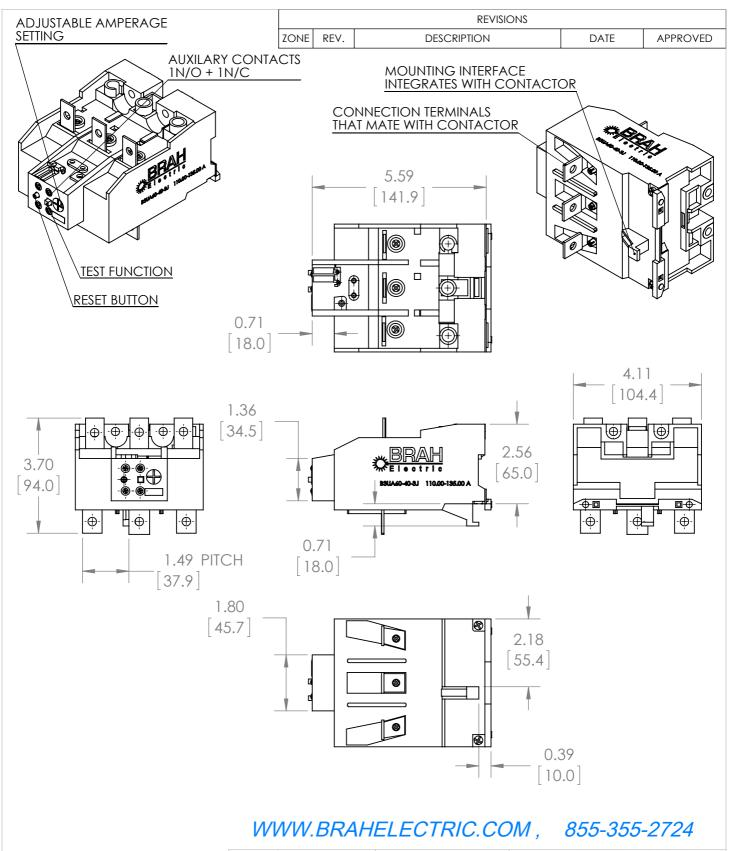
\*NOTE: THIS BRAH ELECTRIC **OVERLOAD RELAY** B3UA60-40-3J AN AFTERMARKET DIRECT REPLACMENT FOR SIEMENS 3UA60-40-3J. SUITABLE FOR USE WITH 3UA MOTOR **CONTROL SYSTEMS**
