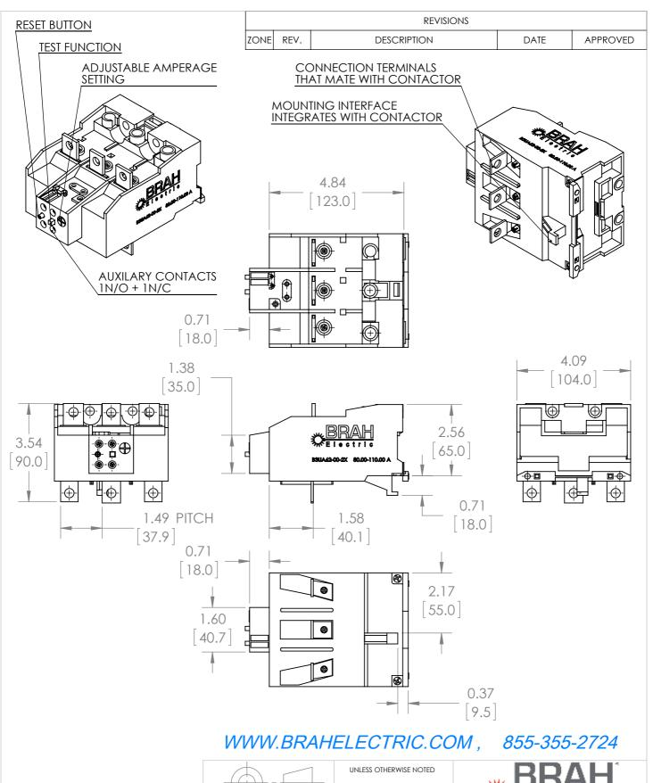
\*NOTE: THIS BRAH ELECTRIC **OVERLOAD RELAY** B3UA62-00-2X AN AFTERMARKET DIRECT REPLACMENT FOR SIEMENS 3UA62 00-2X. SUITABLE FOR USE WITH 3UA MOTOR **CONTROL SYSTEMS**
