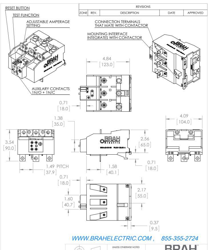
\*NOTE: THIS BRAH ELECTRIC **OVERLOAD RELAY** B3UA62-00-3H AN AFTERMARKET DIRECT REPLACMENT FOR SIEMENS 3UA62 00-3H. SUITABLE FOR USE WITH 3UA MOTOR **CONTROL SYSTEMS**
