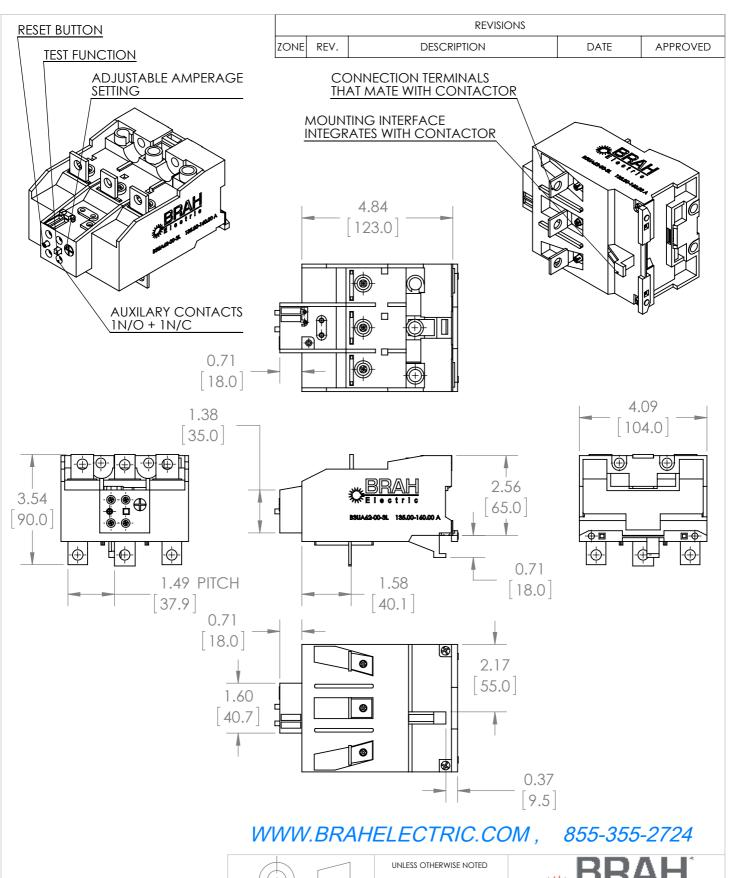
\*NOTE: THIS BRAH ELECTRIC **OVERLOAD RELAY** B3UA62-00-3L AN AFTERMARKET DIRECT REPLACMENT FOR SIEMENS 3UA62 00-3L. SUITABLE FOR USE WITH 3UA MOTOR **CONTROL SYSTEMS**
