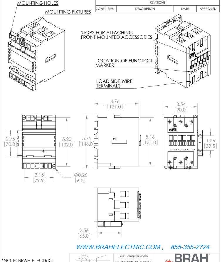
\*NOTE: BRAH ELECTRIC CONTACTOR BA110-30-11-42 IS AN AFTERMARKET DIRECT REPLACMENT FOR A110-30-11-42,A-LINE SERIES. SUITABLE FOR USE WITH A-LINE SERIES MOTOR CONTROL SYSTEMS
