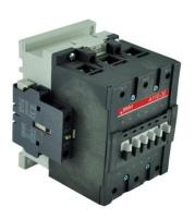
PART NUMBER – BA110-30-11-42: BRAH Electric, aftermarket direct replacement contactors for ABB A110-30-11-42, A-Line series, type A, 3P, 3PH, 110A, 600V, 40HP @ 240V, 75HP @ 480V, 100HP @ 600V, complete with 277V AC coil, and 1 N/O - 1 N/C auxiliary contact, AC magnetic contactor, suitable for use with A-Line series motor control systems
