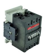
PART NUMBER – BA110-30-11-51: BRAH Electric, aftermarket direct replacement contactors for ABB A110-30-11-51, A-Line series, type A, 3P, 3PH, 110A, 600V, 40HP @ 240V, 75HP @ 480V, 100HP @ 600V, complete with 480V AC coil, and 1 N/O - 1 N/C auxiliary contact, AC magnetic contactor, suitable for use with A-Line series motor control systems
