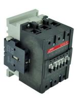
PART NUMBER – BA110-30-11-55: BRAH Electric, aftermarket direct replacement contactors for ABB A110-30-11-55, A-Line series, type A, 3P, 3PH, 110A, 600V, 40HP @ 240V, 75HP @ 480V, 100HP @ 600V, complete with 500/600V AC coil, and 1 N/O - 1 N/C auxiliary contact, AC magnetic contactor, suitable for use with A-Line series motor control systems
